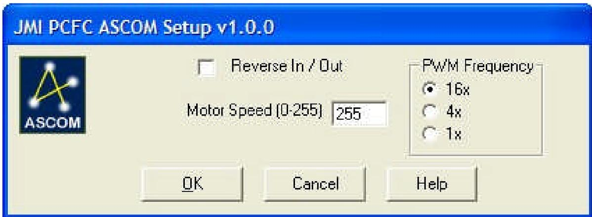
The PCFC ASCOM driver provides a Setup window that allows you to set the motor speed and PWM Frequency as described above. You can also reverse the operation of the motor using the Setup window. The settings you select in the Setup window will be saved and recalled each time you invoke the PCFC ASCOM driver through ASCOM-compliant software.
