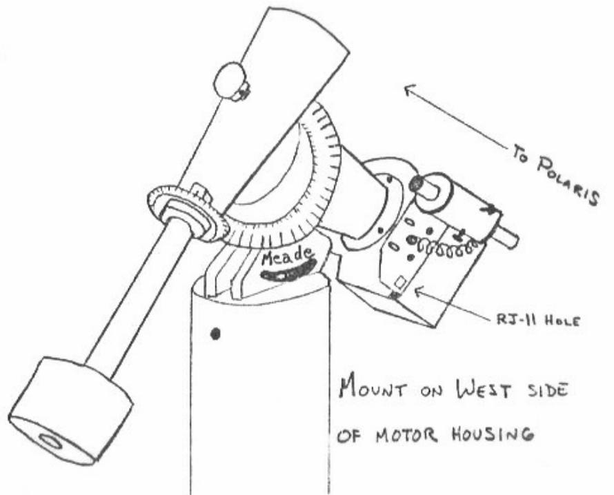
EZAlign Installed on a Meade Equatorial Starfinder
