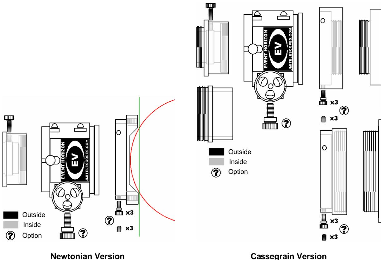
In the diagram above, black lines represent external surfaces, gray lines represent internal surfaces and the question mark shows where you have the option of using metal or nylon thumbscrews or setscrews. Note that the Newtonian version is designed for both flat and curved surfaces. The Cassegrain version shows the output adapters, standard with the EV-1c, EV-2c and EV-3c focusers, and the mounting bases for standard and large-format SCT threads.
