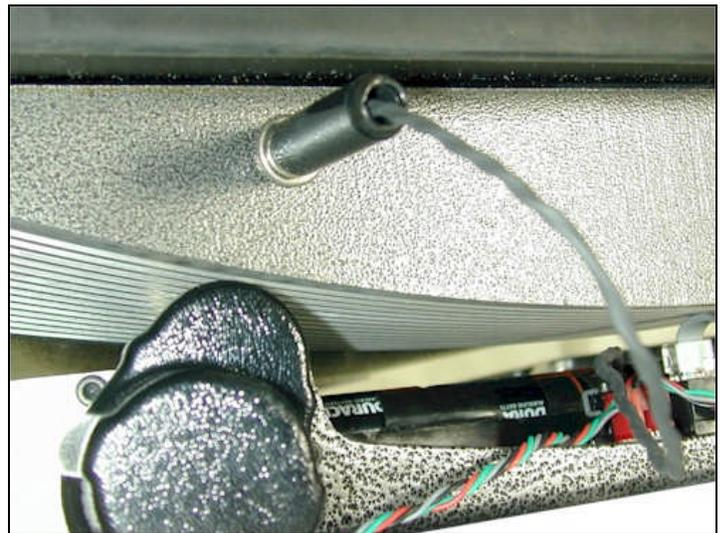
Declination Plug Inserted Into Declination Jack
