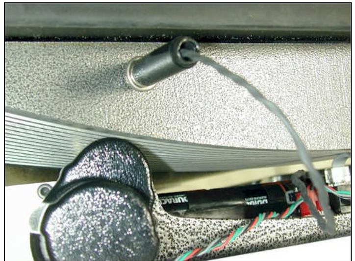
Declination Plug Inserted Into Declination Jack
