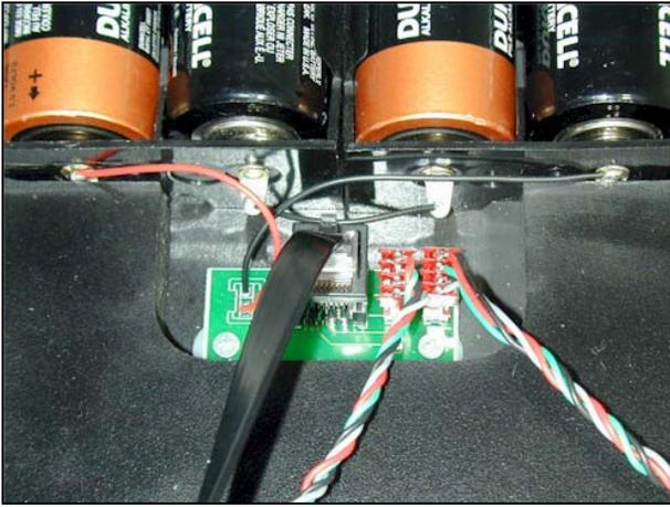
Control (left) and Motor (right) Connectors
