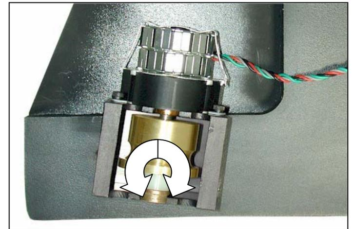
Rotate Brackets to Match Drive Wheels with Plate
